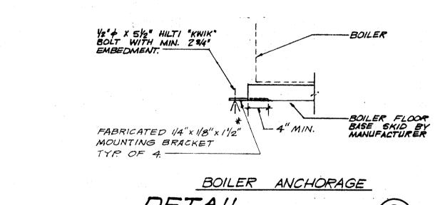
TO PROVIDE SNUG FIT IN BOILER BASE SKID.
