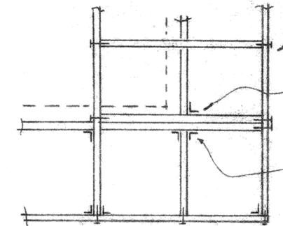
TYP. FRAMING @ ROOF CORNERS (OUTSIDE MODULES) (3)
