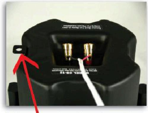
Add your safety wire to this attachment point, as required by local code. Safety wire will support the entire speaker and tile bridge assembly.
